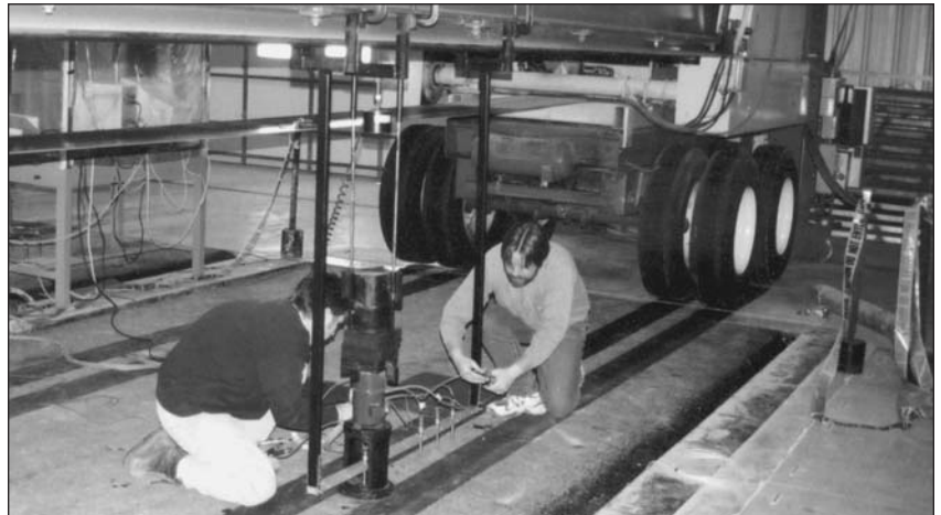
Paul Lewis and student measuring asphalt wear.
