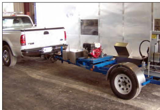
Falling-weight deflectometer tests on completed pavement test sections
