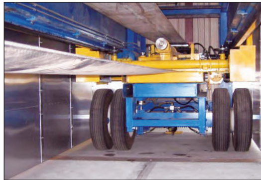
The accelerated pavement test assembly
